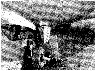
Fig. 5 Early production deflector failure.
